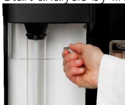
Fig. 2. Closing the Safety door and starting an analysis
